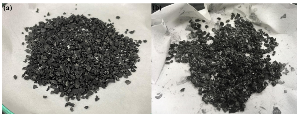
Figure 7. Physical conditions of GAC particles (a) before MP removal and (b) after MP removal.
