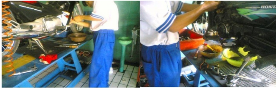
Fig 1. Partial view of working practice in of the workshop motorcycle. Workers are engaged in routine activities without proper personal protective equipment (mask and gloves)
