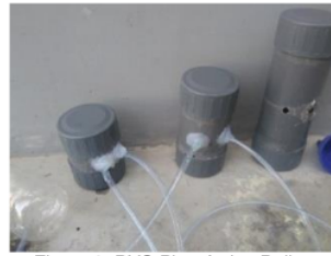
Figure 3. PVC Pipe Active Ballast
