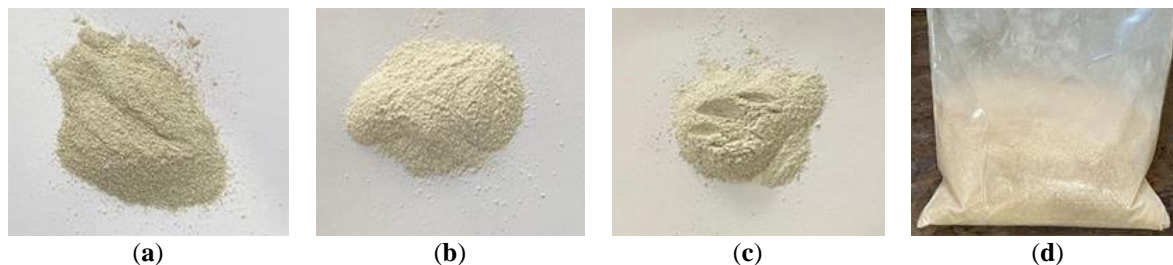
Figure 1. Fishbone powder color after the sintering process: (a) 600 °C; (b) 700 °C; (c) 800 °C; and (d) before the sintering process.
