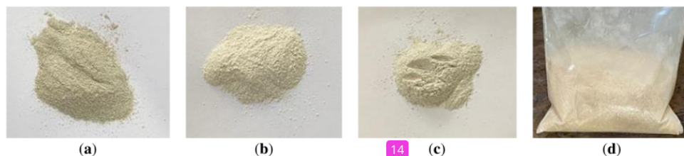
Figure 1. Fishbone powder color after the sintering process: (a) 600 °C; (b) 700 °C; (c) 800 °C; and (d) before the sintering process.
